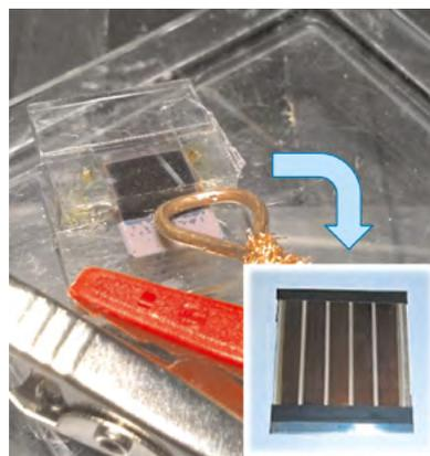
Demo of monolithic back-contact dye solar cells. The goal is to realize a 10 x 10 cm<sup>2</sup> sized sub-module prototype using printing and deposition techniques suitable for roll-to-roll production.
