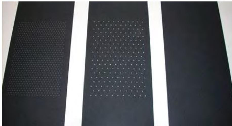
Thermal absorber plates for an unglazed thermal collector prototype
