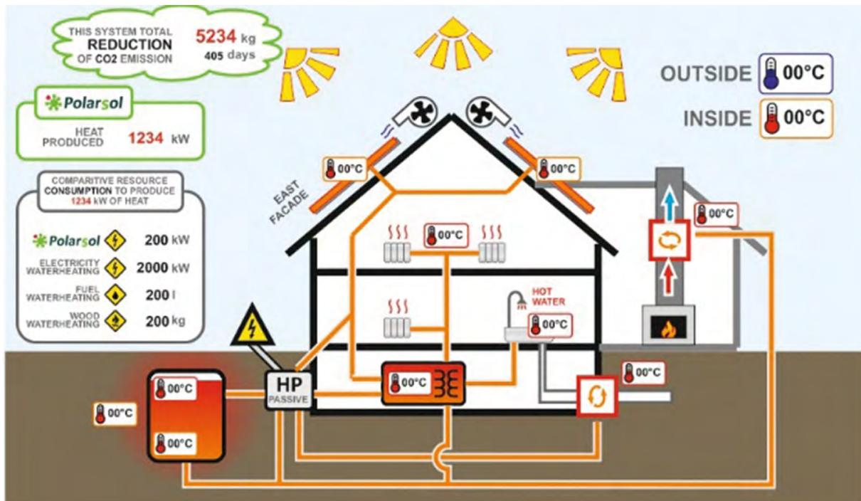
PolarSol solar-thermal heating system
