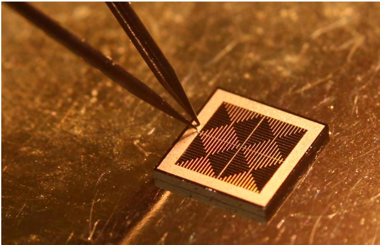
Processed III-V solar cell under test
